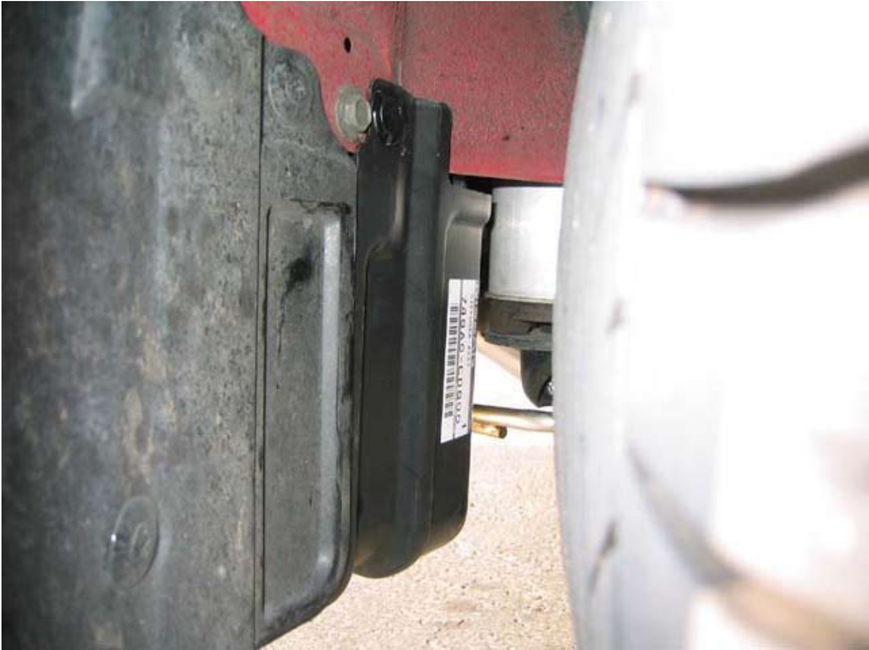
Last picture. Passenger side diffuser installed. View from the side.
